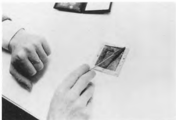
First lifting of masking tape seal
